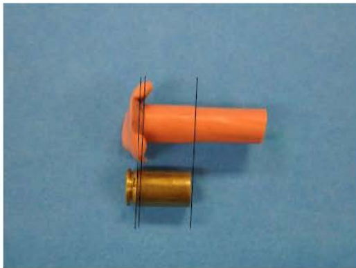
Figure 6-8. Glock 34, 9 mm – Very Small Unsupported Case Wall Area
